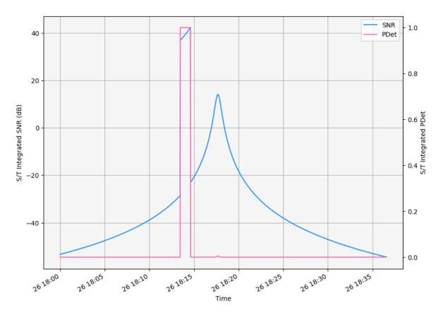
When the private plane flies through the beam, S/T Integrated PDet and SNR (dB) spike. The S/T Integrated SNR (dB) rises as the range between the radar and the aircraft decreases. The S/T Integrated SNR increases in the middle of the graph because the range decreases and the private plane is in a side lobe.
