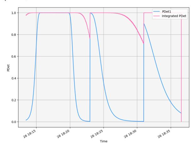
S/T PDet1 uses one pulse and S/T Integrated PDet uses up to 512 pulses. Both S/T PDet1 and S/T Integrated PDet show reflections from the private plane. However, the S/T PDet1 values drop twice, while the S/T Integrated PDet values only drop below 0.8 on two instances.
