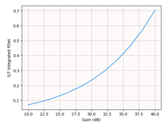
The mean S/T Integrated PDet has a slight increase from a gain of 20 dB through 30 dB. However, from 30 dB through 40 dB there is a steeper climb.
