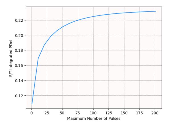
The mean integrated probability of detection has a sharp rise until 50 pulses integrated, after which it begins to level off.
