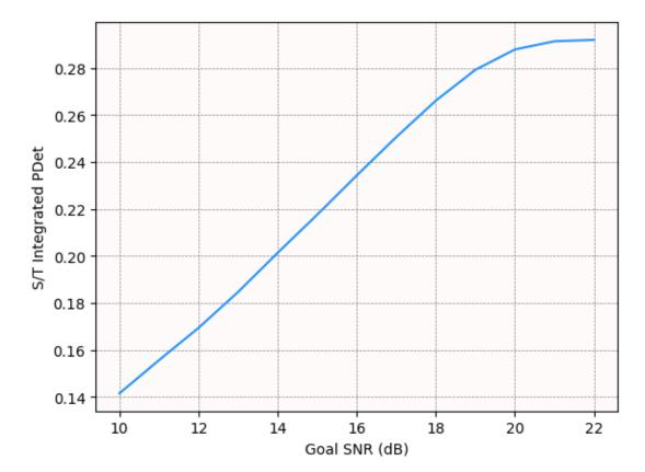
There is a steady increase in mean S/T Integrated PDet until the goal SNR reaches 20 dB. Before continuing to the next trade study, reset the goal SNR to 16 dB:
